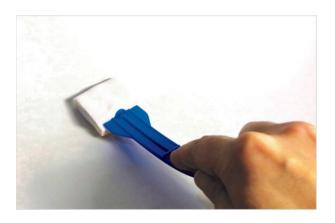
5. With your hands on the outside of the bag, pinch the sponge while turning the EZ Reach handle in a **counter-clockwise** direction one half turn, until it disengages. Discard handle.
