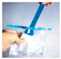
4. After sampling is complete, insert the sponge portion into the original sample bag. Do not insert the handle beyond the central crossing rib, and do not touch the inside of bag with your hand.
