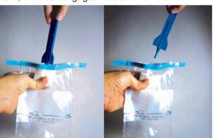
2. Keeping your hands on the outside of the bag, push the EZ Reach handle out of the bag. Grasp the handle above the central crossing rib on the handle and remove sponge sampler from the bag.
